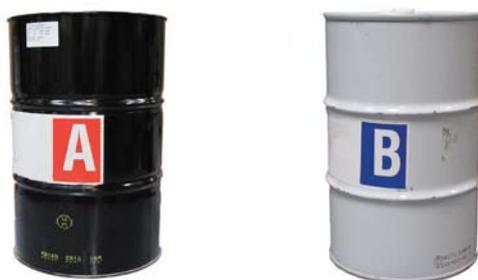
The second kind of SPF is called two-component low-pressure SPF. This product is often used to fill in large cracks and crevices, and it is also used with special PPE. This second kind of product is primarily used by professionals doing home weatherization and other trained workers. If the visual media content depicts chemicals in a kit or box containing two cylinders or what look like small propane tanks, it will be a two-component low-pressure type of foam.
